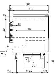
Drain Electrical inlet (power)
